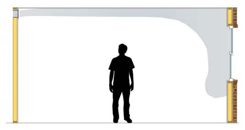
Figure 4. High sidewall supply outlet example
