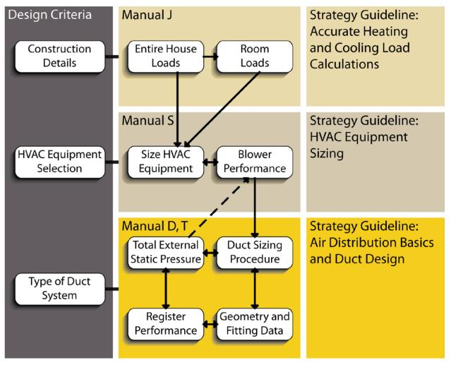
Figure 1. HVAC design flow
