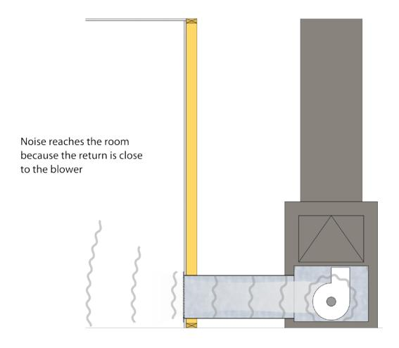
Figure 7. Return placement introduces noise
