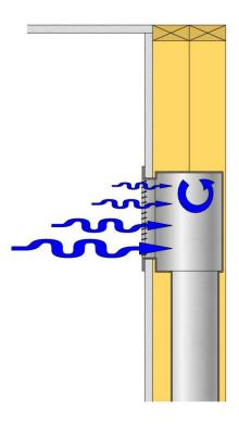
Figure 18. Poor return grille placement
