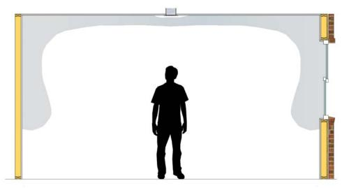
Figure 5. Ceiling supply outlet example
