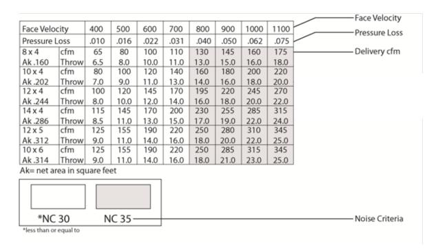
Figure 22. Example supply outlet performance data
