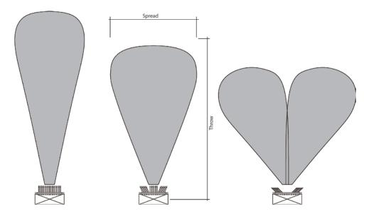
Figure 6. Example throw and spread of air outlets
