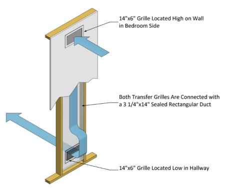
Figure 16. High/low through-the-wall transfer grille
