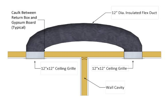
Figure 17. Attic transfer duct
